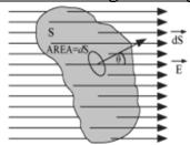
For calculating total flux through any given surface, divide the surface into small area elements. Calculate the flux at each area element and add them up.
