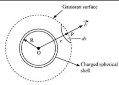
Let  $\vec{E}$  be the electric field at point P. Then, the electric flux through area element  $\vec{d}$  is given by,  $d\phi = \vec{E} \cdot \vec{d}$  is
