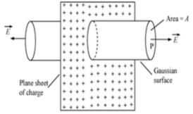
Let P be the point at a distance 'r' from the sheet at which electric field is required. Draw a Gaussian cylinder of area of cross-section A through point P.
