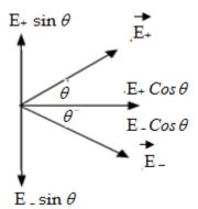
If we resolve  $E_{+q}$  and  $E_{-q}$  each into two perpendicular compents as in figure . The components normal to the dipole axis cancel away. The components along the dipole axis add up.
