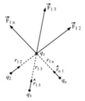
Consider that n point charges  $q_1$ ,  $q_2$ ,  $q_3$ , ...  $q_n$  are distributed in space in a discrete manner. The charges are interacting with each other. Let the charges  $q_2$ ,  $q_3$ , ...  $q_n$  exert forces  $\vec{F}_{n_2}$ ,  $\vec{F}_{n_3}$ ,
