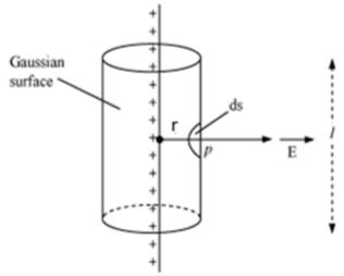
If *E* is the magnitude of electric field at point P, then electric flux through the Gaussian surface is given by,
