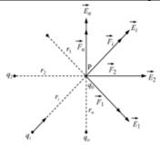
Consider that n point charges  $q_1$ ,  $q_2$ ,  $q_3$ , ...  $q_n$  exert forces  $\vec{F}_{12}$ ,  $\vec{F}_{13}$ , ...,  $\vec{F}_{1n}$  on the test charge placed at origin O.
