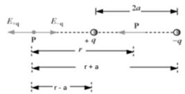
Let P be at distance r from the centre of the dipole on the side of charge q. Then,
