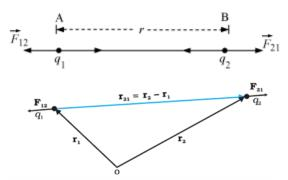
Consider two likecharges  $q_1$  and  $q_2$  present at points A and B in vacuum at a distance r apart. According to Coulomb's law, the magnitude of force on charge  $q_1$  due to  $q_2$  (or on harge  $q_2$  due to  $q_1$ ) is given by,
