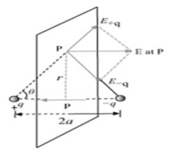
Therefore  $E_{+q}=E_{-q}$ The directions of  $E_{+q}$  and  $E_{-q}$  are as shown in the figure.
